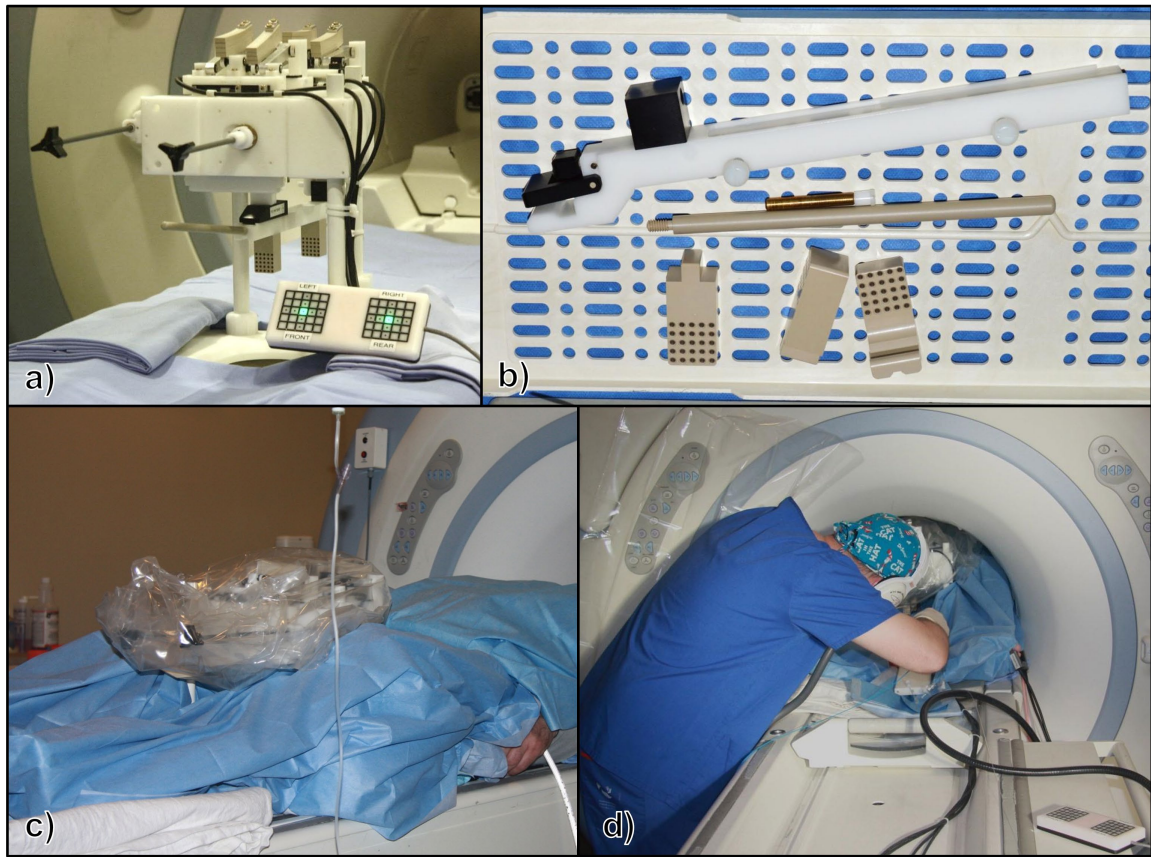
Figure 4.1: Needle guidance device setup and components. a) Device in place on MR table prior to patient positioning. LED grid panel indicates position of the needle guide relative to target position. b) Sterilizable components including (from top to bottom): guidance arm, mounting pin, alignment handle and needle guides. c) Device in operating position before moving the patient into the MR bore. d) Placement of laser fibers with the patient remaining inside the bore.
